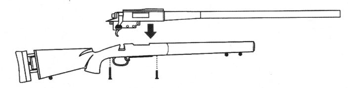
When assembling the replica, pay extra attention to the proper positioning of the screws- the shorter one is designed in the hole closer to the muzzle, the longer screw is designed into the hole between the trigger guard and the stock.
